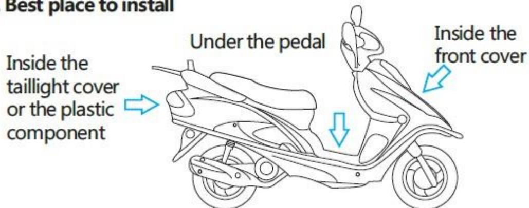
NOTE: The GPS signal will be attenuated if the device is installed under the driver seat.
