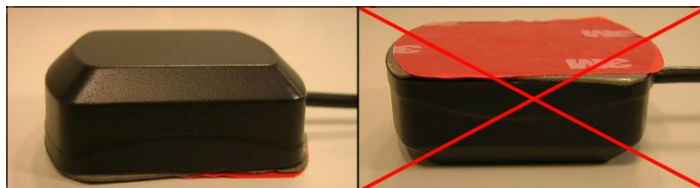
Figure 59. Correct GNSS antenna mounting
